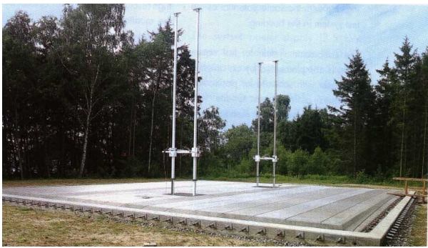
Fig. 1 Open area antenna test site of BAPT in Itzehoe with its two 8 m high antenna rigs
