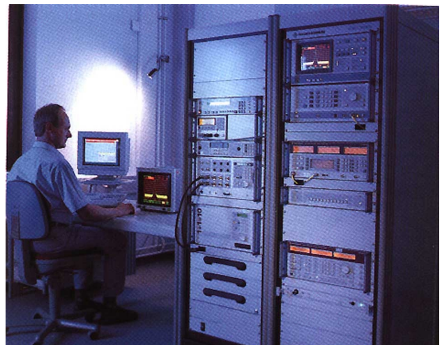
FIG 2 Germany's first standard-conformant antenna calibration system at BAPT in Itzehoe
